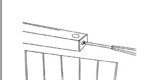
1: From the centre pivot line of the hinges, measure 222mm and secure the guide roller to the gate. This will line up with the locating marks which are on the body of the closer.
